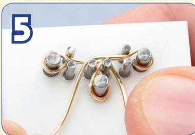
Continue with the same wire back across the form and bend the wire down between the two pegs as shown.
