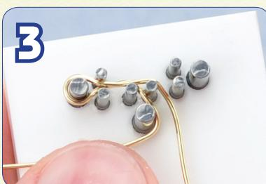
Continue by moving the wire back across to the right and down between the two pegs as shown.
