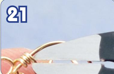
Use the flush cutter once again to remove the end of the wire.
