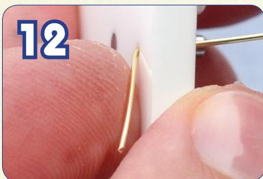
Insert the end of wire (20-24Ga) 7" in length into the hold in the Findings Form, then bend the end down as shown.
