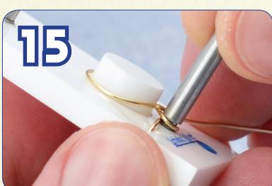
Use the pusher tool to flatten the wires around the peg.
