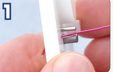
Insert a piece of wire (20-24Ga) 5" (12.7 cm) in length through the hole in the Findings form and bend the end (this helps to hold the wire firmly as you bend the wire around the pegs).
