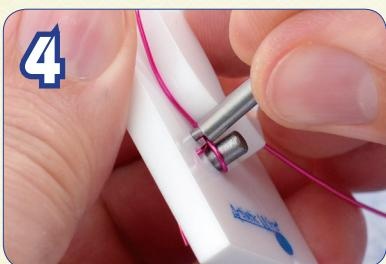
Use the Pusher tool on the small peg to tighten the intersection of the wire.
