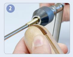
Use as a wire guide with the Coiling Gizmo. As the wire passes through the clamped leather tips, it gets an additional straightening just before it is wound onto the mandrel.
