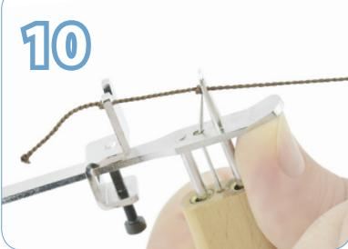
Continue pulling the Silk down with the left hand to keep tension on the knot, and push up with the thumb of your right hand on the knotter tool so the tool will push the knot up and off the awl delivering the knot at the specified length away from the other knot.
