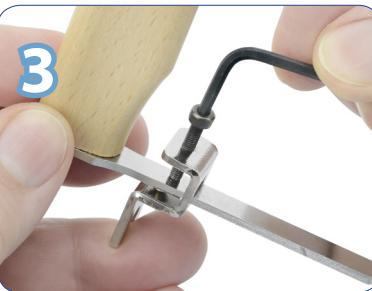
Tighten the Allen Set Screw with the included Allen Wrench, make sure the movable extender is the proper distance before final tightening.
