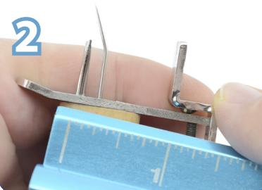
Measure the desired knot length from the yoke on the Knotter Tool (near the Awl), to the yoke on the movable extender.
