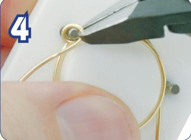
Carefully cut 1/4 of the loop off using the flush cutters with the flush portion facing the ring that will stay on the form.
