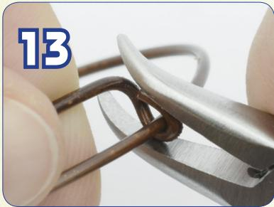
Rotate the wire form and pliers to close the tip of the loop. Leave ample room for the wire to move freely inside of the newly closed loop.
