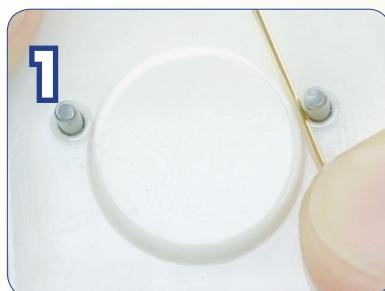
Place the end of the wire between the form and the right peg as shown. Hold in place against the jig with your thumb.
