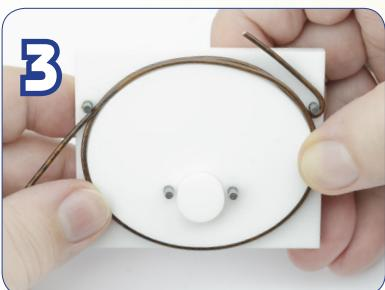
Hold down the two wires and wrap the long wire around the form counter-clockwise for one full revolution. Continue to wrap the wire around and in between the form and the peg on the left.
