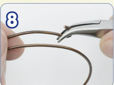
Grasp the loop as shown with Bent Chain Nose Pliers, make sure with larger gauges of Wire that you have a good grasp on the wire for the bend.
