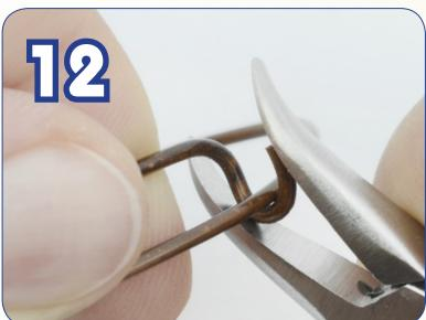
Using the Bent Chain Nose Pliers, carefully close the loop part of the way.
