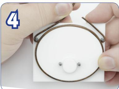
Wrap the end of the wire clockwise around the left peg to match the other wire around the right peg.
