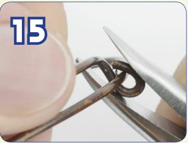
Follow steps 12 & 13 to securely close the second loop. Make sure there is ample room for the wire to move freely within the loop.
