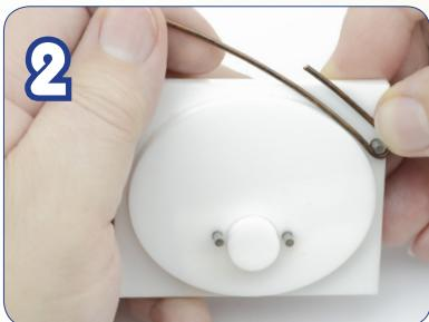
Bring the short end of the wire around the peg counter-clockwise until it is parallel with the other wire.
