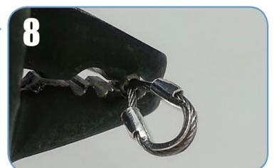
10. With the rounded portion of the crimper tool, close a crimp bead cover over the crimp bead.
