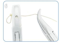
Place a Nylon Jaw Pliers against the coil and hold the end of the Wire with Chain Nose Pliers.
