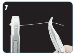
7. Slowly pull the Wire to the right while holding the Nylon Jaw Pliers firmly against the coil.
