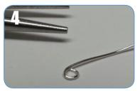
8. Reposition the pliers within the loop to finish the loop.
